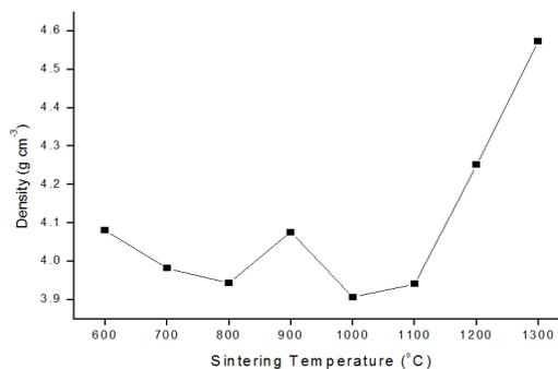
**Figure 2: Density of BNT Ceramic with  $x=0.15$  at Different Sintering Temperature**
