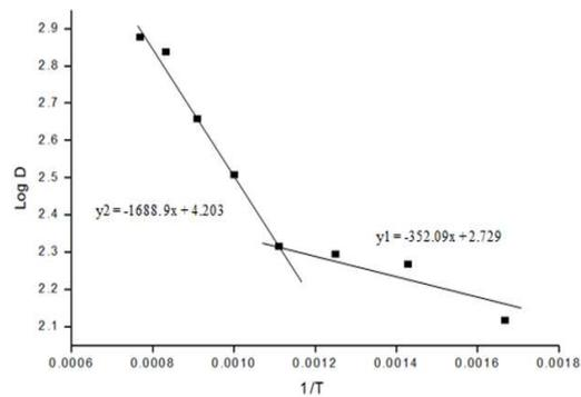
**Figure 5: Activation Energies of Grain Growth**
