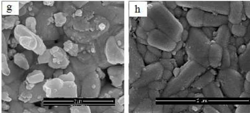
**Figure 4: Microstructure of BNT Ceramic for All Sintering Temperatures; (a) 600°C, (b) 700°C, (c) 800°C, (d) 900°C, (e) 1000°C, (f) 1100°C, (g) 1200°C, and (h) 1300°C**
