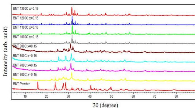
**Figure 1: XRD Pattern of BNT Ceramic with  $x=0.15$  for All Sintering Temperatures**
