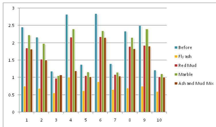
Figure 1: Comparative Fluoride Concentration before and after Using Adsorbents in Phase I
