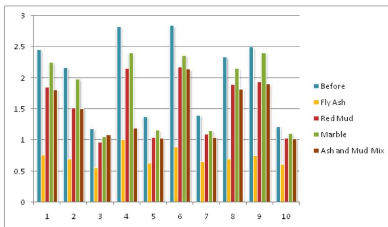
Figure 3: Comparative Fluoride Concentration before and after Using Adsorbents in Phase III
