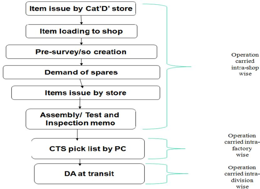
**Process 2: Issue to Instrument Shop to Repair and Overhaul Completion, Testing and Dispatch**
