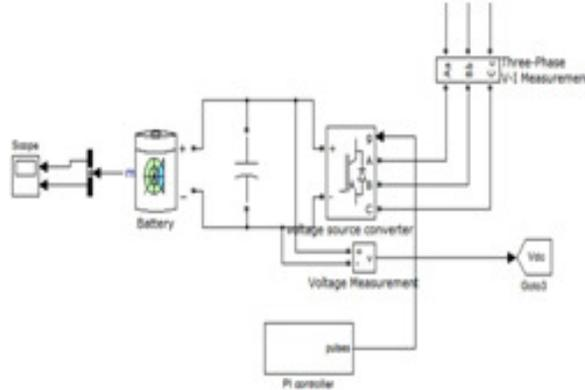
Figure 5: Voltage Source Inverter with Battery and Controller
